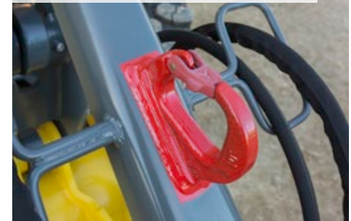
Load hook on the tilt rod (standard)
