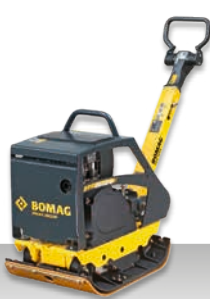
BPR 25/40 D Operating weight: 150 kg Centrifugal force: 25 kN Working width: 400 mm
