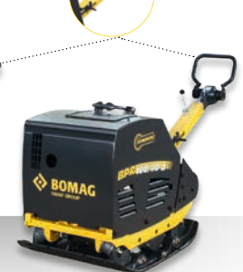
BPR 100/80 D Operating weight: 710 kg Centrifugal force: 100 kN Working width: 800 mm
