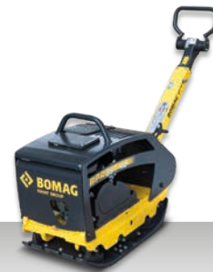
BPR 35/42 Operating weight: 190 kg Centrifugal force: 35 kN Working width: 420 mm
