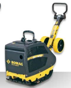
BPR 35/42 D Operating weight: 210 kg Centrifugal force: 35 kN Working width: 420 mm
