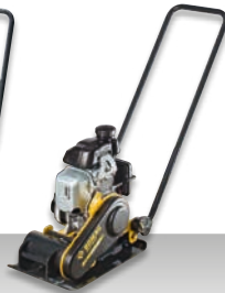
BVP 10/30 Operating weight: 47 kg Centrifugal force: 10 kN Working width: 300 mm
