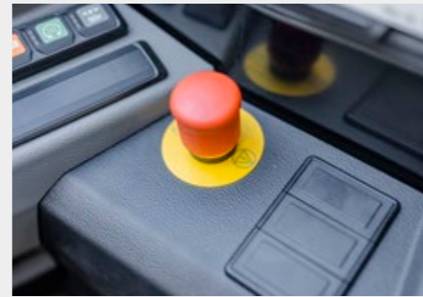
Quick to reach emergency switch so that the machine can be immediately moved into a safe state in an emergency.
